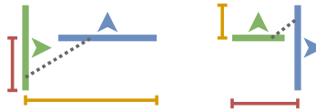
Figure 3.2: Quads q shown in blue can see p shown in green with the dotted line being a possible view ray between them. The arrows indicate their orthogonal facings in 2D. The AABBs for such aligned quads are flat and have no volume. The descent b_k^q - b_k^p > 0 of p into H_q is marked in red while the ascent b_j^q - b_j^p > 0 of q into \bar{H}_p is marked in orange. Viewing this scene in 3D simply extrudes the quads without changing the content.
